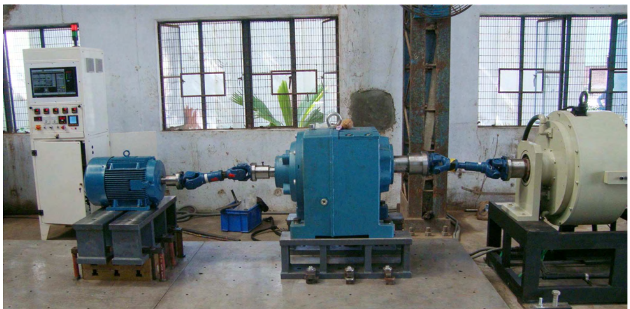
10000 Nm Powder Dynamometer for Gear Box Test .
