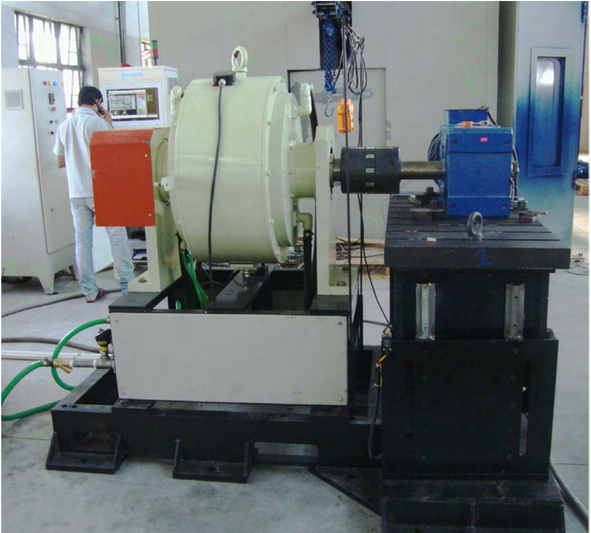
10000 Nm Powder Dynamometer for Gear Box Test .
